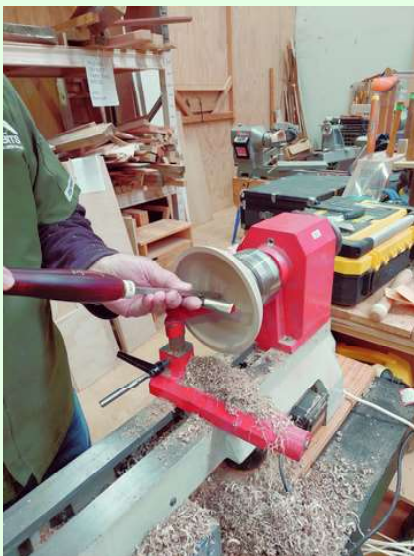
Mark demonstrating techniques for hollowing out a bowl on his portable lathe.
